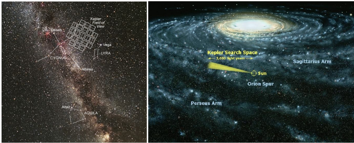
Figure 2.6: Left: Field of view of the Kepler space telescope projected onto the night sky. Each rectangle marks one of the 42 CCD detectors. The constellations Cygnus, Lyra and Aquila (the primary stars of which form the well-known “summer triangle” in the northern hemisphere) are also shown. Right: Artists impression of the Milky Way galaxy, indicating the position of our solar system and the search space covered by observations with Kepler . Note that the distance marked corresponds to the magnitude range of observed main-sequence stars. Image Credit: Carter Roberts and Jon Lomberg.
